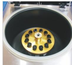
Vacuum port is on the center of rotor to make contamination to be minimized.
