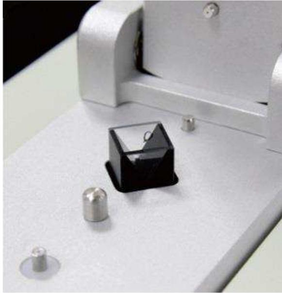
**√ Unique designed pipette holder for easy sample adding**
